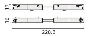
After inserting into the track, rotate the lock counterclockwise to fix the conduction and load bearing fixation!
